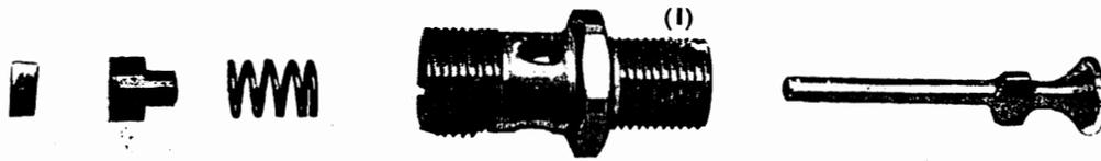
FIG. 57 — CLAPET DE DÉMARRAGE DÉMONTÉ
