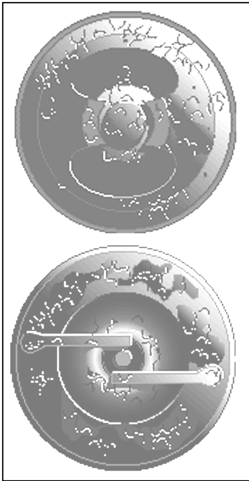
FIGURE 8-6. Typical carbon-fouled spark plug.
